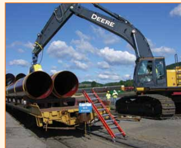
A hydraulic suction crane unloads Transco pipes to be used in the construction of natural gas lines. Transco ships its pipes on the LVRR from its facility in South Avis.
