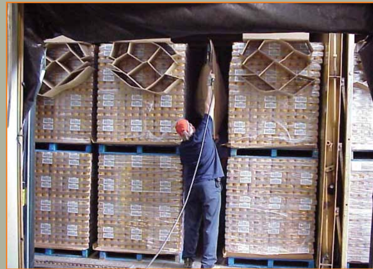
A pneumatically inflated airbag creates a bulkhead that minimizes load movement. This is just one method used to prevent freight damage.
